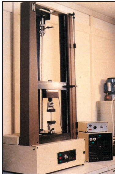
This tensile testing machine measures the effects of a force applied to a fixed test specimen and is also used in a compression mode for testing conventional door and window seals, as well as intumescent seals.
